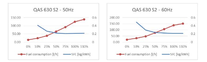
(Reference conditions at 25°C Air Inlet Temperature, 60% Relative Humidity, 1bar Absolute inlet pressure, for different conditions or limitations contact Atlas Copco technical support).
