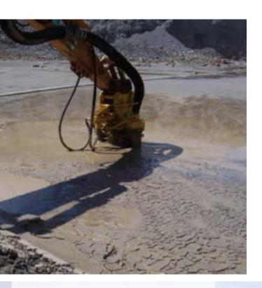
Hydromining offers a superior alternative to loading and hauling unwanted material.
