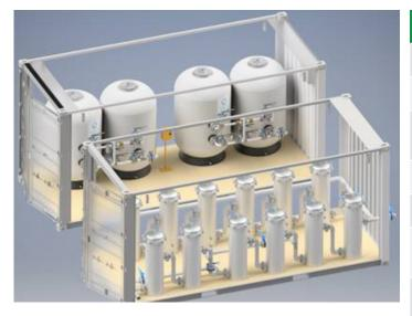
The P2 Unit is a granular-media-based filtration system that houses four filter vessels in two separate stages. The unit is employed exclusively in PFAS treatment trains, as the final polishing step. The vessels can be run in two configurations: four filters in series, or two parallel trains of two filters each. Which configuration is used will depend on flow rates and incoming water quality.
