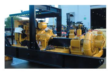
Fuel Consumption: 53 L/hr @ BEP 900rpm WMR Fuel Capacity: 3000 litres, 24hrs @ 1200rpm
