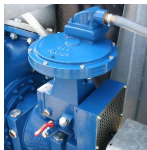
Priming system Diaphragm pump, air-cooled, water-resistant and oil-spillage free. Air capacity of 50 m 3 per hour.
