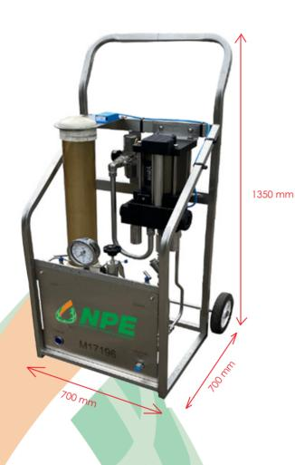
The air-driven high-pressure pumps used in the chemical injection unit are particularly built for maximum performance and efficiency. The device has been developed for both on and offshore operations and is housed in 316 Stainless Steel trolley for portability.
