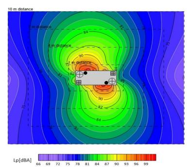
The test is done at 75% of the prime power at 60Hz
