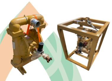
Air driven/pneumatic/diaphragm pumps are specifically designed for optimum performance and efficiency. They are driven by the well-known positive displacement pump technology.
